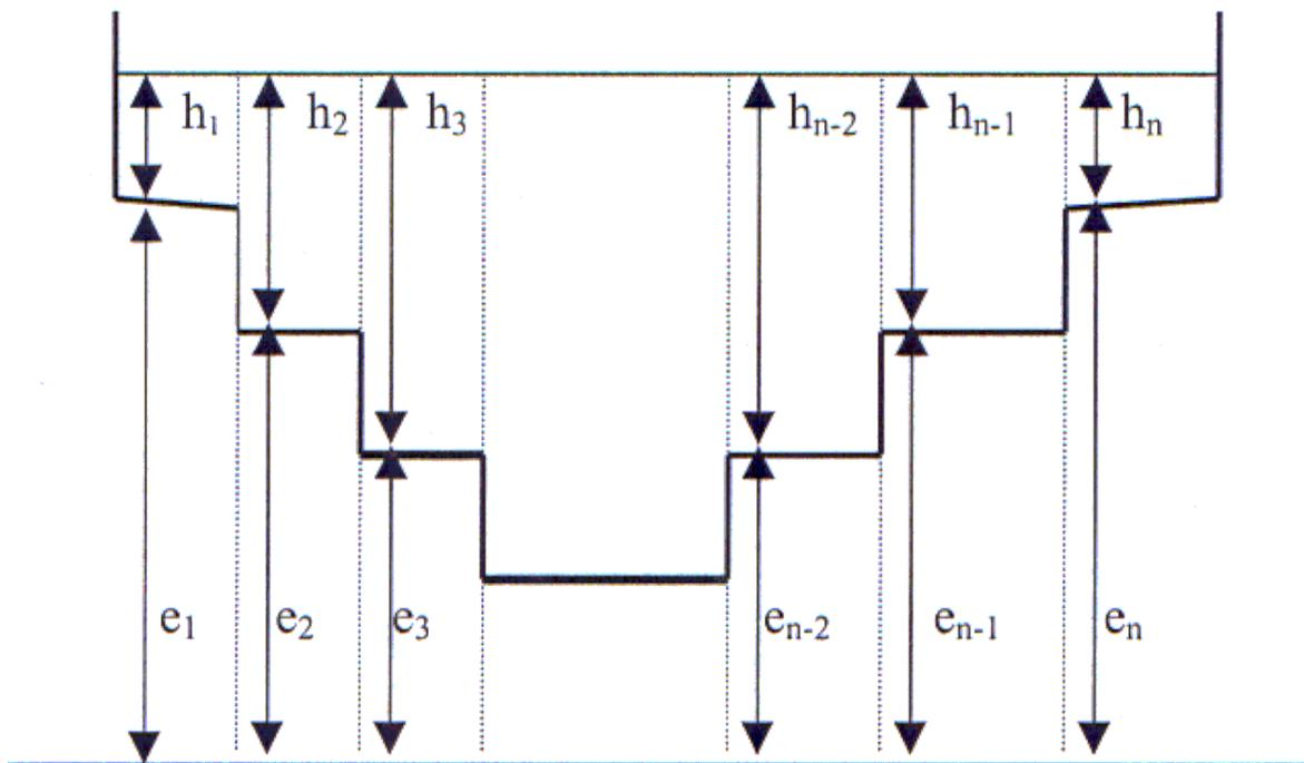
Figure 4: Discretization of a fluvial cross-section
