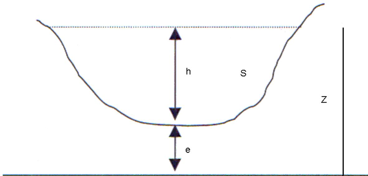
Figure 3: A one-dimensional fluvial cross-section
